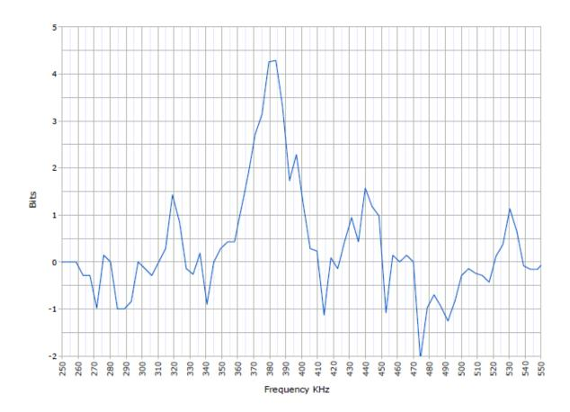
The amplitude is the number of bits the spectrum is reduced when the crosstalk is present.
